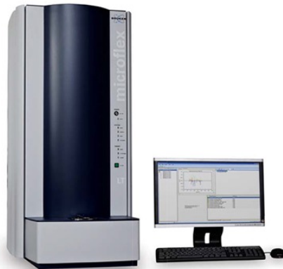
MALDI Biotyper microflex-NID1 (Bruker Daltonics, Germany)
