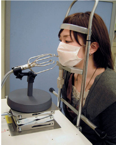
Fig. 1. Measuring the speed of the wind from the mouth with an ultrasonic anemometer. The anemometer/thermometer sensor was placed in front of the mouth. The subject in this picture wore a paper mask.
